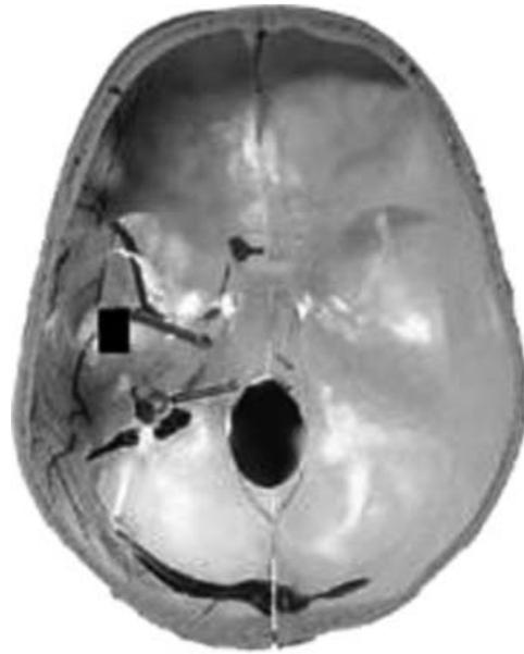
Fig. 5. Location of the strain gage rosette attached to the inside of the skull above the mandibular fossa.
