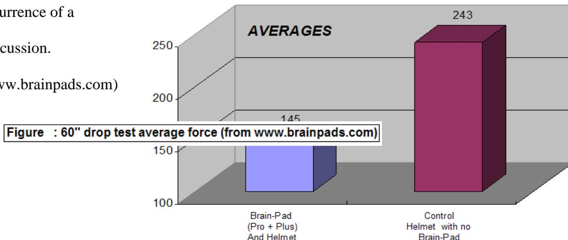
Figure : 60" drop test average force (from www.brainpads.com)
